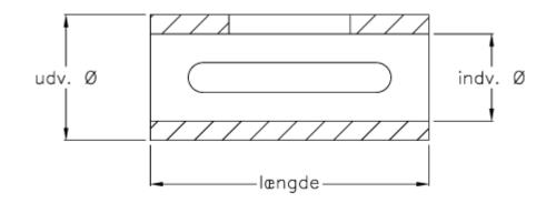
Description = 11/19Internal diameter = 11Length = 35Outer diameter = 19
